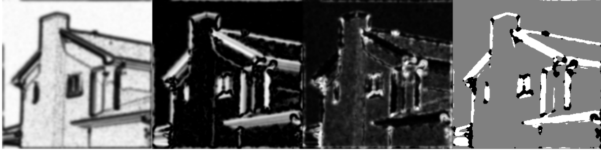
Figure 3. Computed iD for the image in figure 2, black means zero and white means one. From left to right: c_{i0D} , c_{i1D} , c_{i2D} and highest confidence marked in gray, white and black for i0D, i1D and i2D, respectively.
