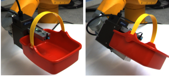
Figure 11. The robot is doing a rotation to extract the 3D model of a basket.
